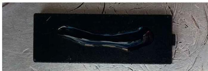
5. To ensure the tag stays in place a decent amount of 2-part epoxy should be used. If coated too sparingly the tag will not remain in place. Bond strength is increased with heat.
