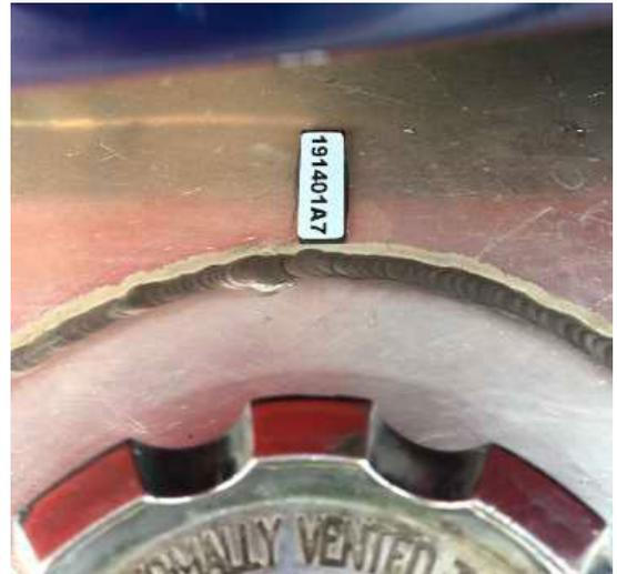
When vertical, the tag can be placed below steps and cabin overhangs without a significant impact to read ranges.
